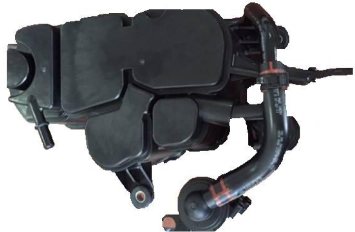
Multi canister design incorporating various grades of activated carbon for gasoline vapor recovery
